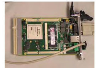
LEON3FT Eval. Board (Rad-Hard, SpW, High MIPS / Watts ratio)
