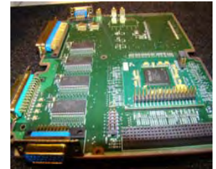
SCIF Board (H/W framer, RAM-based S/W I/F; Transitioned to RBSP)
