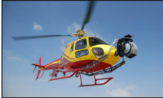
Conducted flight test of flash lidar sensor for Altair's autonomous landing and hazard avoidance
