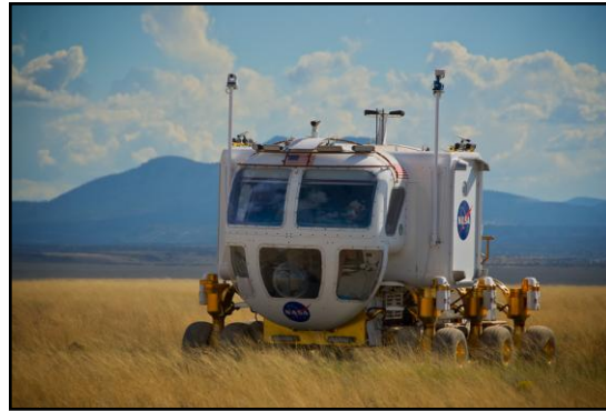
Demonstrated Lunar Electric Rover and suit-port concept for enabling travel beyond the lunar outpost.
