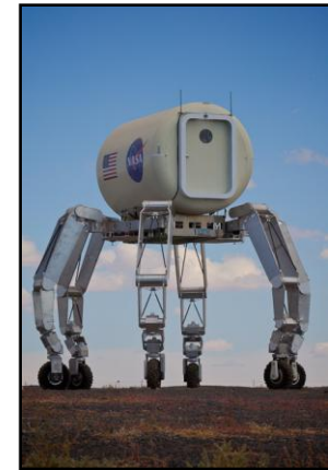
Demonstrated Tri-ATHLETE rover for unloading habitat module from lunar lander
